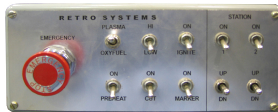
Operator control panel with process and UP / DOWN switches and E-STOP button.
