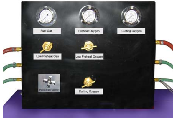
Hi / Low Preheat Gas Control Panel with Ease-On Pierce Rate Control
