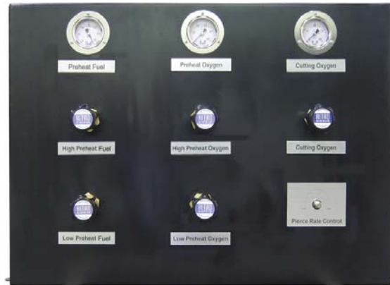
Hi / Low Preheat Gas Control Panel
