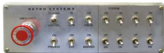
Operator control panel for (4) stations
