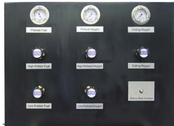
Hi / Low Preheat Gas Control Panel
