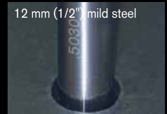
12 mm (1/2") hole without True Hole technology
