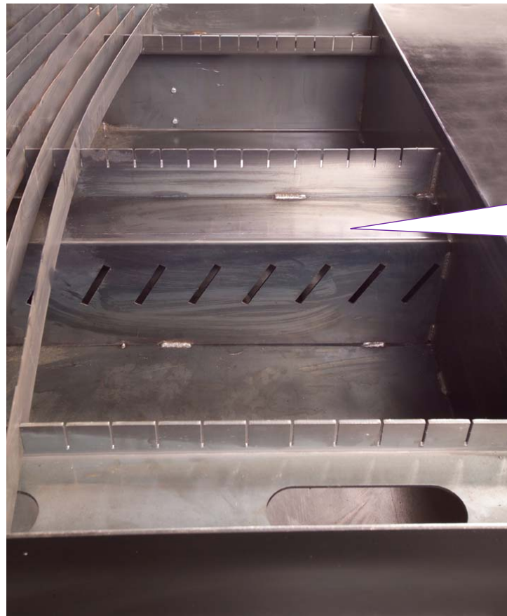
Air table with salts removed to show Center Exhaust Tube
