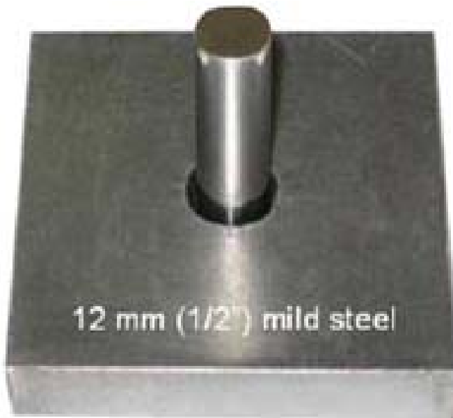
12mm hole cut in 12mm steel without TRUE HOLE™ Technology
