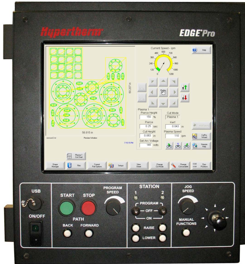
EDGE Pro CNC control with version 9 software to support TRUE HOLE™ technology
